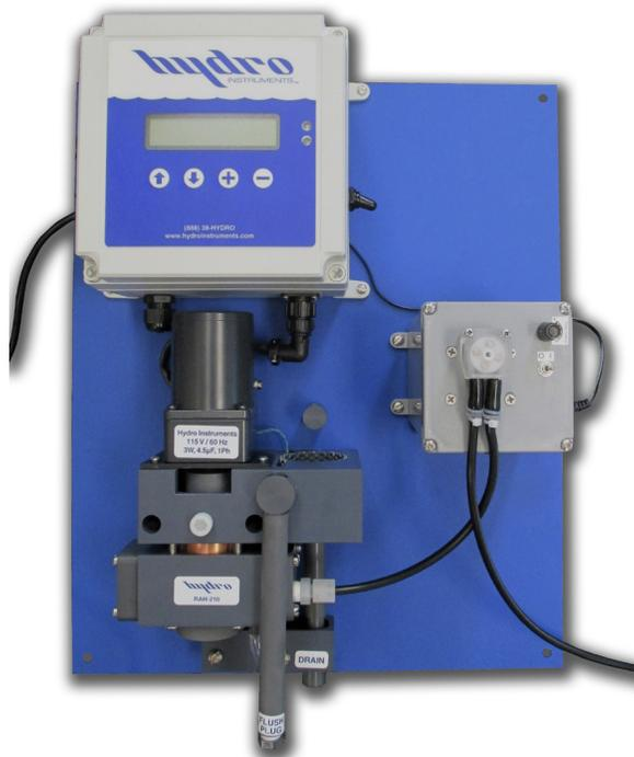
The Series RAH-210 Analyzer makes use of the Amperometric method to determine residual levels in the sample water. The measurement cell consists of large anodic and cathodic electrodes in direct contact with the sample water. The measurement is continuous, not relying on sample and hold methods, thereby allowing for better process control. A continuously driven cleaning system is employed to prevent the build up of impurities on the surface of the electrodes and reduce the need for maintenance.
